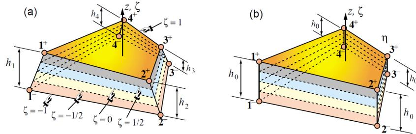
Figure 1: Wall fabrication assumption for solid shell element. (a) constant thickness, (b) variable thickness. [4]
